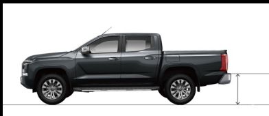
Cargo Box Floor Height: 820mm
