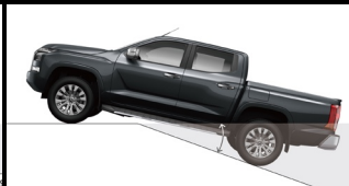
Ramp Break - Over Angle: 23.4deg
