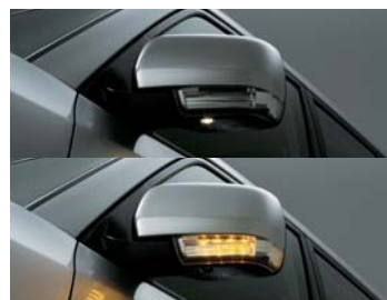
Chrome power door mirrors with approach lamps and turn lamps 📷 10
