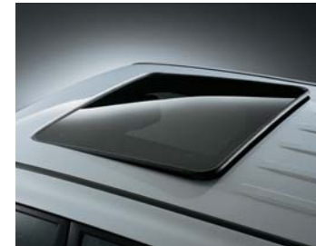
Power tilt and sliding sunroof with anti-trapping function 📷 17
