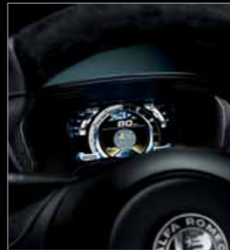
Full digital instrument panel with TFT technology Carbon fibre instrument panel fairing
