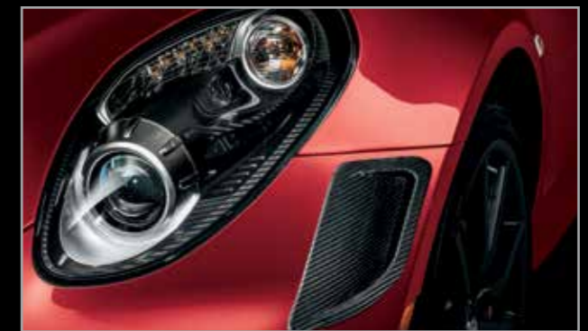
Bi-Xenon headlights and front bumper with carbon fibre intake
