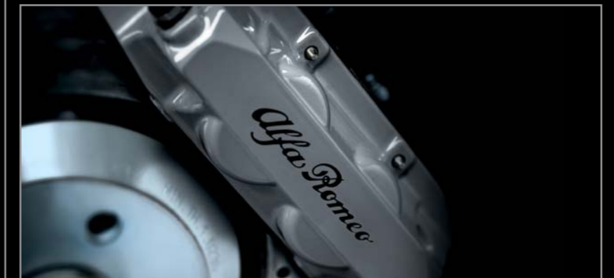
Dual-cast, perforated, self-ventilated, 305x28 mm front discs with Brembo fixed 4 piston calipers
