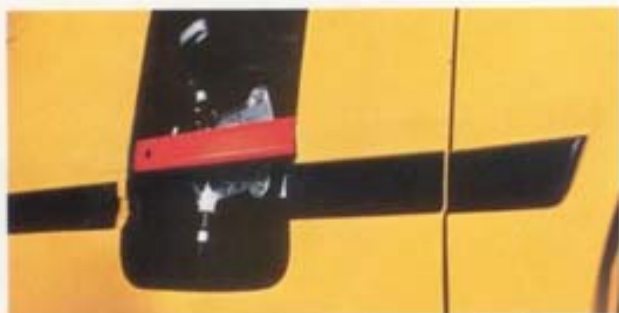
A sturdy rod framework in the doors can double the resistance in certain side-collisions.
