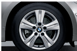
□ 2BT 16" light alloy Double-spoke style 222 with 205/55 R16 tyres (standard on SE models).
