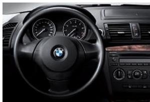
■ Standard steering wheel , three-spoke (diameter 375mm).
