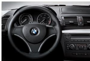
□ 255 Three-spoke Sport leather steering wheel (diameter 369mm).
