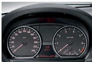
■ Instrument cluster with analogue instruments and red backlighting: speedometer, LC display for mileage counter, trip counter and On-Board Computer, plus rev counter with integrated fuel gauge.
