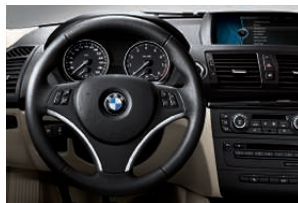
□ 249/255 Sport multi-function leather steering wheel, three-spoke (diameter 369mm), includes controls for radio and factory-fit telephone (standard on SE models).
