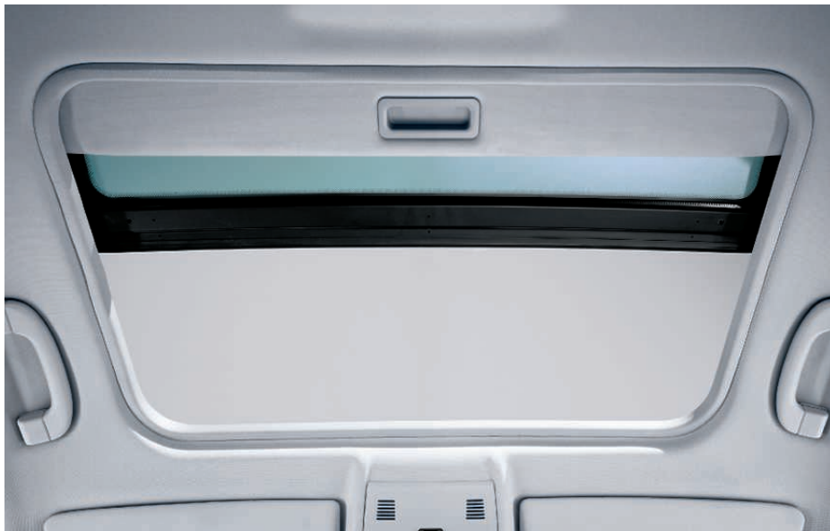
□ 403 Glass sunroof with sliding and tilt function electric adjustment can also be operated via the key.
