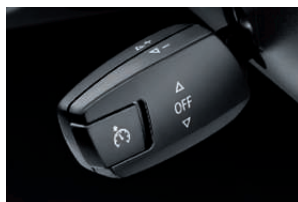
□ 540 Cruise control stores and maintains a desired speed above approx. 20mph activated using the left-hand steering-column stalk. After accelerating, the vehicle automatically returns to the previously stored speed. Braking cancels the setting.
