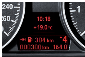
■ On-Board Computer , including the following functionality: fuel consumption and range, information display-analogue instruments combined with liquid crystal display and personal profile functions.
