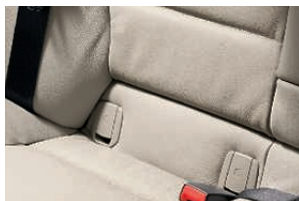
■ Child seat ISOFIX attachment anchorage points are located on the two rear outer seats and front seat (with airbag deactivation). This allows a child seat to be secured safely using its integral snap-on latches.
