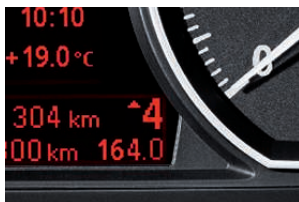
■ Optimum Shift Indicator for models with six-speed manual transmission. The display indicates when you could be driving more economically in a different gear. The system recommends when to shift up or down and adapts its recommendations to your driving style.
