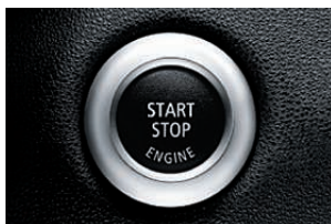
■ Start-Stop button for the engine. Once you've inserted the ignition key, you can start and stop the engine by pressing this button.
