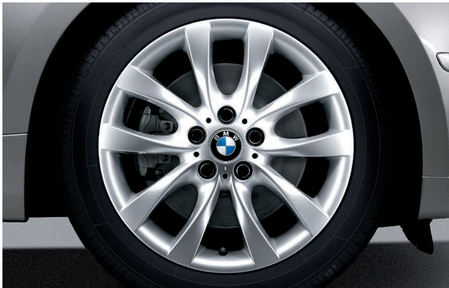
□ 2KF 18" light alloy V-spoke style 217 with 205/45 R18 front, 225/40 R18 rear tyres.
