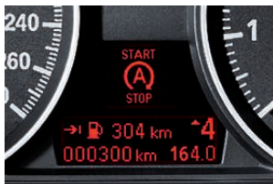
■ Auto Start-Stop indicates on the Info Display when Auto Start-Stop has switched off the engine, at traffic lights, for instance. The display switches off again when the engine is restarted automatically (for all models in conjunction with six-speed manual transmission). Also indicates when system is not active due to external conditions.
