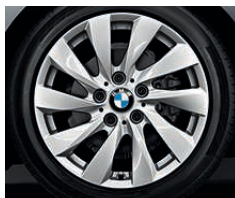
2AS 17" light alloy Turbine-spoke style 381 , with 7.5J x 17 with 225/45 R17 run-flat tyres.
