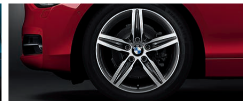
■ 2DT 17" light alloy Star-spoke style 379 , in Orbit Grey and burnished metal, 7.5J x 17 with 225/45 R17 run-flat tyres.
