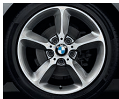
2DU 17" light alloy Star-spoke style 382 , in Space Grey and burnished metal, with mixed tyres; front 7.5J x 17 with 225/45 R17, and rear 8J x 17 with 245/40 R17 run-flat tyres.
