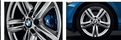
□ 2NH M Sport braking system, oversized brake discs – front and rear, Blue painted brake calipers with 'M' designation. (Included within M Sport Plus package).
