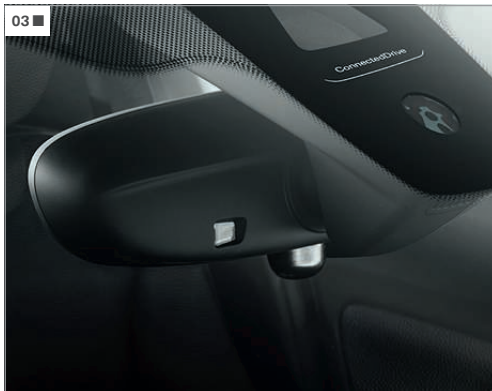
[ 03 ] The rain sensor including automatic headlight activation automatically switches on the windscreen wipers and the low-beam headlights.
