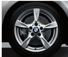
□ 2DM 17" light alloy Star-spoke style 371 with run-flat tyres, 7J x 17" with 205/50 R17 tyres (standard with Exclusive Edition models).
