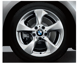
□ 2AP 17" light alloy Streamline-spoke style 370 with mixed run-flat tyres, 7J x 17" with 205/50 R17 tyres at the front, 7.5J x 17" with 225/45 R17 tyres at the rear.
