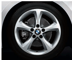
□ 2R2 17" light alloy Star-spoke style 256 with run-flat tyres, 7 J x 17 with 205/50 R17 tyres (standard for SE models), also available as a complete winter wheel set from the Genuine BMW Accessories range.
