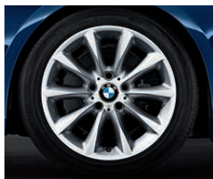
□ 2DH 17" light alloy Star-spoke style 340 with mixed tyres, 8 J x 17, 225/45 R17 tyres at the front, 8.5 J x 17, 255/40 R17 tyres at the rear (standard on 335i SE).
