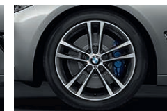
□ 2V5 19" light alloy M Double-spoke style 598 M with mixed run-flat tyres, front 8J x 19 with 225/45 R19 tyres, rear 8.5J x 19 with 255/40 R19 tyres. (Standard with M Sport Plus package).
