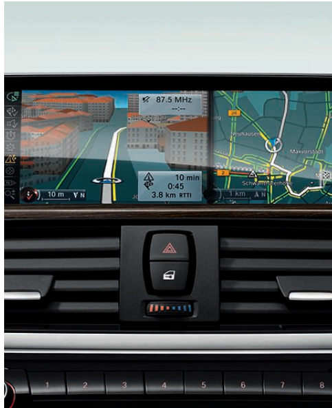
□ 609 Navigation system – BMW Professional , including high-resolution 8.8" display, DVD changer, latest generation iDrive Touch Controller with direct access buttons, favourites, integrated hard disk (20GB) for audio data and navigation instructions, 3D city models, multi map views and Real Time Traffic Information (RTTI). 1
