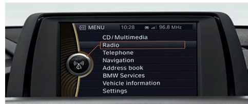
■ BMW Professional radio , includes a 6.5" colour monitor, iDrive Controller with direct menu control buttons, a CD drive and MP3 decoder.
