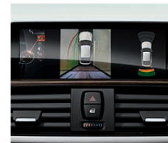
□ 5DL Surround-view includes Top-view and Side-view cameras, and enables a wide field of visibility. This system enhances parking and manoeuvring in confined spaces as well as increasing visibility when joining a road from a side street.
