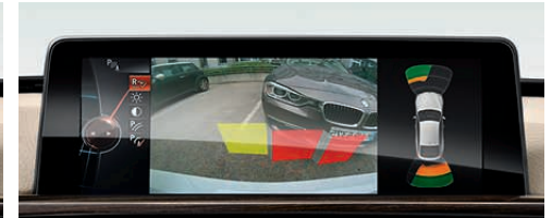
□ 3AG Reversing Assist camera shows a clear image of the area behind the vehicle on the Control Display. In addition, the rear view camera enhances visibility when reversing and parking.
