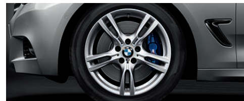
■ 2PE 18" light alloy M Star-spoke style 400 M with mixed run-flat tyres, front 8J x 18 with 225/50 R18 tyres, rear 8.5J x 18 with 255/45 R18 tyres.
