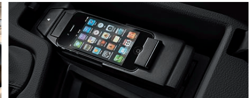
□ 6NS Enhanced Bluetooth telephone preparation, USB audio interface and Voice Control , for wireless in-vehicle connection of suitable Bluetooth mobiles 4 . Audio devices such as an MP3 player, iPod or USB stick can be connected via the integrated USB interface.
