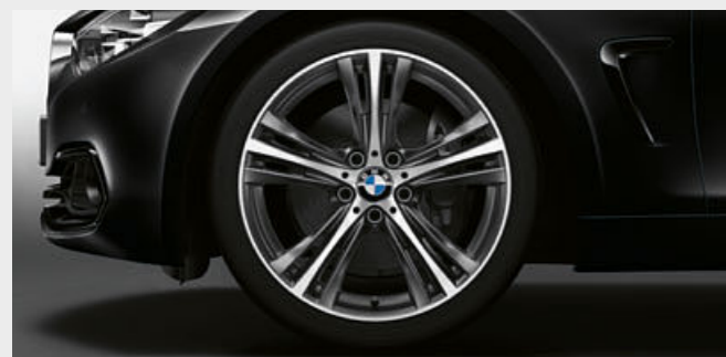
■ 19" light alloy Star-spoke style 407 wheels, Bicolour Orbit Grey with mixed run-flat tyres, front 8J x 19 with 225/40 R19 tyres and rear 8.5J x 19 with 255/35 R19. Optional for Sport models.
