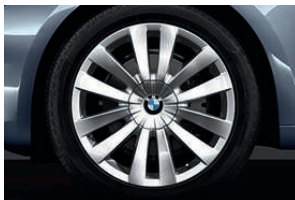
□ 2BX 20" light alloy Double-spoke style 253 with mixed tyres, 8.5J x 20 wheels and 245/40 R20 run-flat tyres at the front, 10J x 20 wheels and 275/35 R20 run-flat tyres at the rear.
