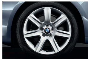
□ 2SW 19" light alloy Star-spoke style 272 with mixed tyres, 8.5J x 19 wheels and 245/45 R19 run-flat tyres at the front, 9.5J x 19 wheels and 275/40 R19 run-flat tyres at the rear (standard on 550i SE).
