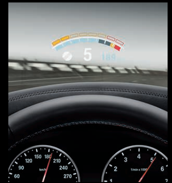
The M specific Head-Up Display shows additional driver information like the optimal gear-change point.
