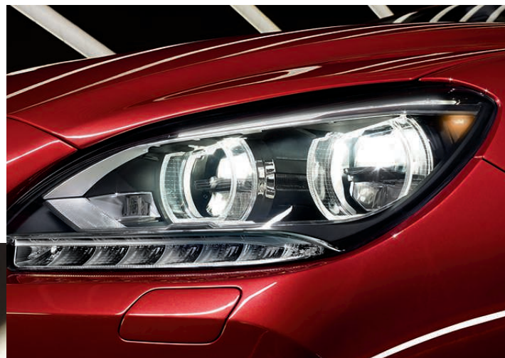
Low and high beams can be generated by optional LED technology. As with the Adaptive turning lights, the headlights follow the course of the road and adapt their beam to the traffic conditions.
