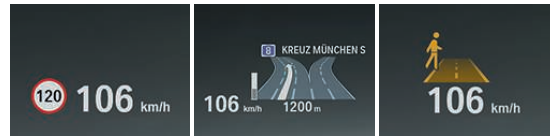
Seen from the driver's point of view, the Head-up Display appears to hover above the vehicle's bonnet.
