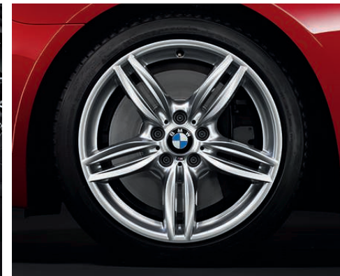
19" M light alloy Double-spoke style 351M with mixed tyres, front 8.5J x 19" with 245/40 R19 tyres, rear 9J x 19" with 275/35 R19 tyres.
