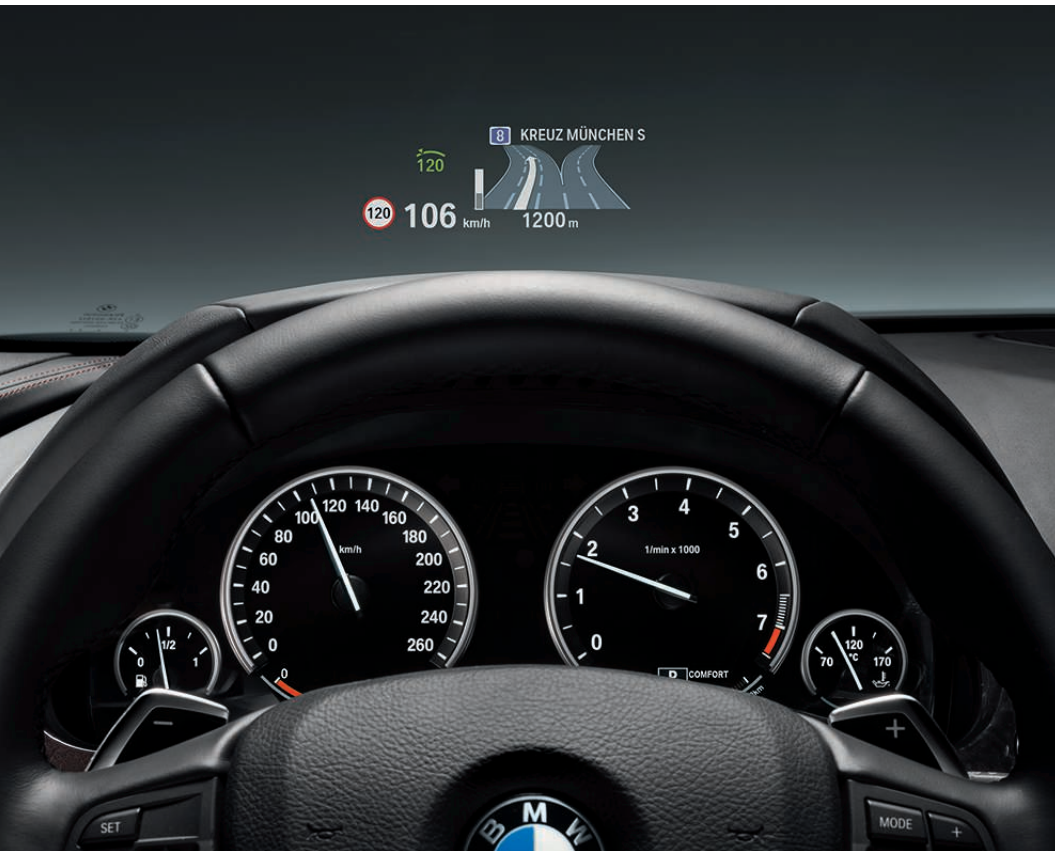
Seen from the driver's point of view, the Head-up Display appears to hover above the vehicle's bonnet.
