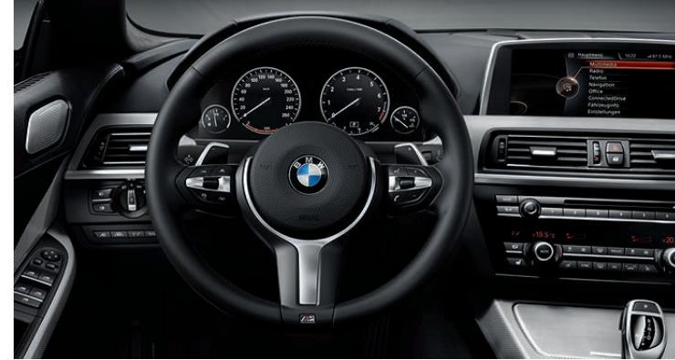
M Sport multi-function leather steering wheel, with multi-function buttons and gearshift paddles.
