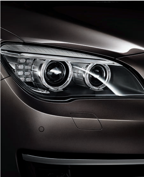
■ Xenon Headlights for high and low beam, including automatic headlight range control and headlight washing system for significantly better illumination of the road at night or in poor light. □ 524 Adaptive Headlights with variable light distribution, including cornering lights for better illumination of road ahead through corners.
