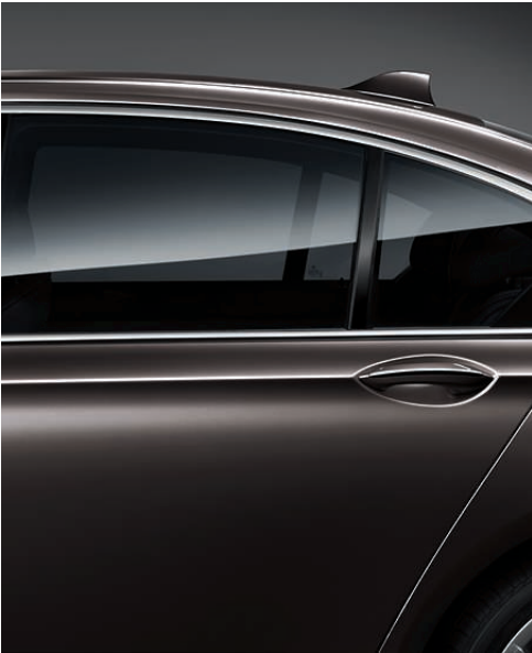
□ 356 Climate comfort laminated glass for the rear side windows (from the B-pillar) and rear window. The tinted glass reduces glare and ensures a cooler cabin during hot weather. (Standard on 760Li models).
