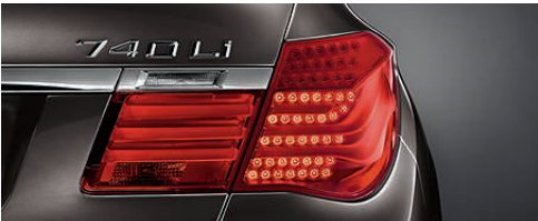
■ Brake Force Display. For even greater safety, these help vehicles following behind to see how hard you are applying the brakes. During normal braking, they illuminate in full. In emergency braking, they start to flash.
