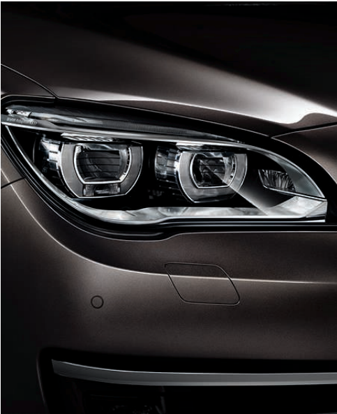
□ 552 Adaptive LED Headlights for high and low beam, includes High-beam Assistant, adaptive turning lights, cornering lights, side indicators and accent light with LED technology. Full 'white' headlights offer greater resemblance to daylight for excellent visibility. Emitted via four Corona rings making the headlights unmistakable day and night.
