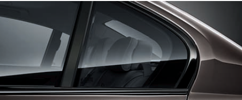
■ Exterior trim High-gloss Shadowline includes window recess covers and window frame trim in high-gloss Black (standard on M Sport models).
