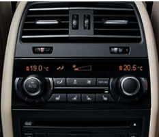
■ Air conditioning, automatic with four-zone control, separate temperature controls for driver and front passenger plus the temperature in the rear can be adjusted individually via two rotary switches with display. Includes automatic air recirculation, microfilter, humidity solar sensor and max cool button.
