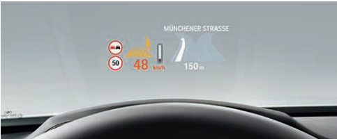
□ 610 Head-up Display, in full colour, delivers driving-related information, such as speed, directly into the driver's field of vision. All information can be projected in full colour making it even easier to recognise.
