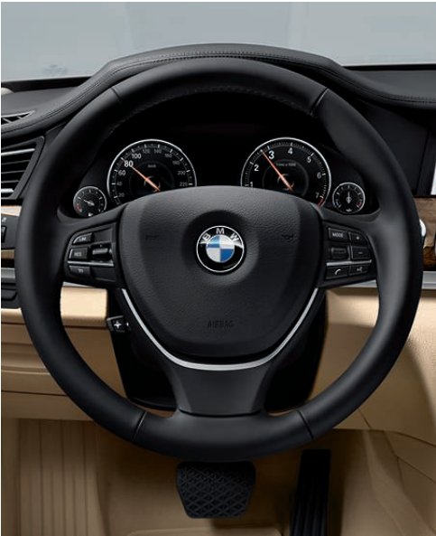
□ 255 Sport leather steering wheel with multi-function buttons sits comfortably in the hands thanks to the thicker rim and sculpted grip sections. The integrated buttons ensure safe control of telephone, voice and audio functions as well as Cruise Control. (Not available on M Sport models). □ 2TE Steering wheel gearshift paddles.
