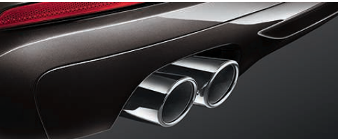
■ Tailpipes: the 730i/Li, 730d/Ld and ActiveHybrid 7 models are fitted with twin round tailpipes on the left.
