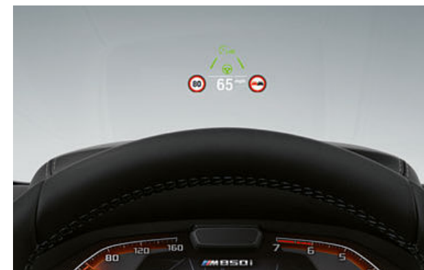
THE BMW HEAD-UP DISPLAY TRANSMITS RELEVANT DRIVING INFORMATION INTO THE DRIVER'S LINE OF VISION WITHOUT DISTRACTION.
