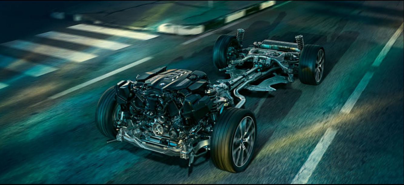
THROUGH THE ADAPTIVE M SUSPENSION PROFESSIONAL WITH BODY ROLL STABILISATION AND THE LATEST-GENERATION BMW xDRIVE, THE BMW M850i COUPÉ IS COMFORTABLE AND ALSO EXCEPTIONALLY SPORTY.
