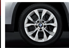
■ 17" light alloy V-spoke style 318 7.5J x 17" with 225/50 R17 tyres.
