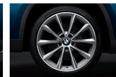
□ 2FN 19" light alloy V-spoke style 324, 8J x 19" with 225/40 R19 front and 9J x 19" with 225/35 R19 rear run-flat tyres.
