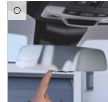
This innovative vehicle interior mirror incorporates an adaptive universal remote control for up to three garage doors and property gates.
