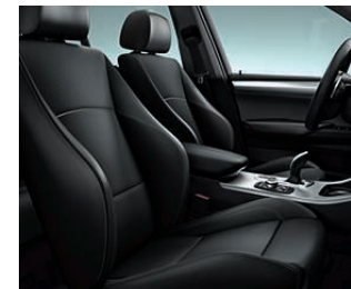
Sport seats, front in Nevada leather upholstery with manual adjustment for fore & aft position, height, recline, thigh support pad, seat tilt and headrests. Enhanced lateral support via pronounced seat bolsters and electric adjustment of seat backrest width.
