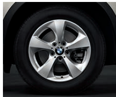
2AM 17" light alloy Streamline style 306 , 8 J x 17 with 245/55 R17 run-flat tyres.
