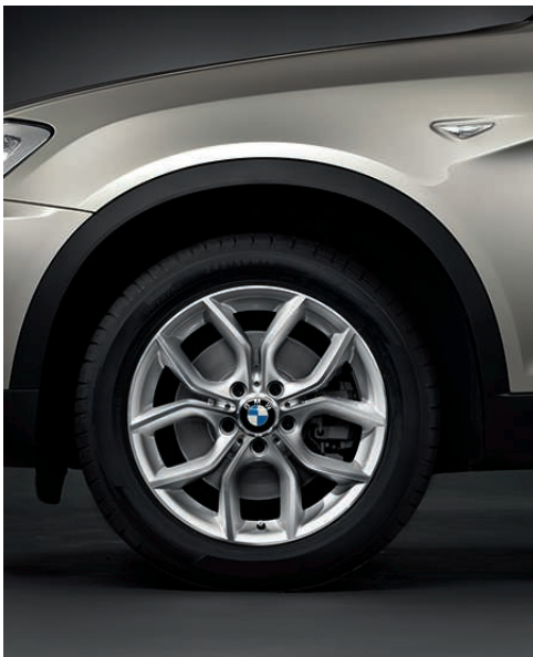
2EC 18" light alloy Y-spoke style 308 , 8 J x 18 with 245/50 R18 run-flat tyres.
