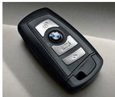
328 Comfort Access for opening and locking the vehicle without holding the key.
