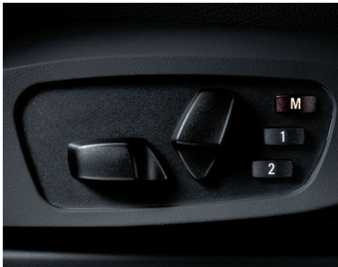
459 Seat adjustment , electric for all front seat parameters, and manual adjustment of steering column.
