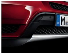
Titanium insert on front bumper. Both outside air vents in the front bumper have a titanium-look panel surround.
