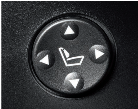
488 Lumbar support for driver and front passenger seats, electrically adjustable for height and depth, for an ergonomically perfect seat position and support of back muscles.
