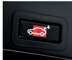
316 Tailgate operation, automatic. Automatic tailgate operation via the remote key. Closing is instigated by a button on the inside of the tailgate. Opening is via an electro-hydraulic mechanism.
