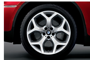
□ 2LE 20" light alloy Y-spoke style 214 , 10 J x 20" wheels at the front with 275/40 R20 tyres, 11 J x 20" wheels at the rear with 315/35 R20 tyres. (Available in optional 2RV Black).
