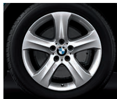
2SH 19" light alloy Star-spoke style 258 with mixed run-flat tyres: 9J x 19 with 255/50 R19 tyres at the front, 10J x 19 with 285/45 R19 tyres at the rear (available in conjunction with Dynamic package).
