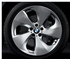
2AL 20" light alloy Streamline style 297 with mixed run-flat tyres, 10J x 20 with 275/40 R20 tyres at the front, 11J x 20 with 315/35 R20 tyres at the rear.
