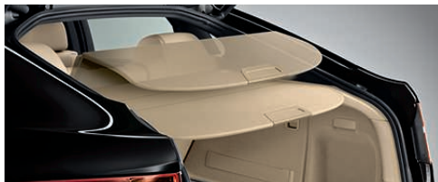
■ Luggage compartment cover , foldable, can be easily detached and stored under the luggage compartment floor.
