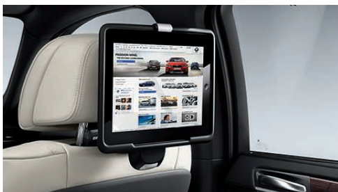
Travel comfort system base carrier with Apple iPad 1 holder attaches to front headrest support bars.
