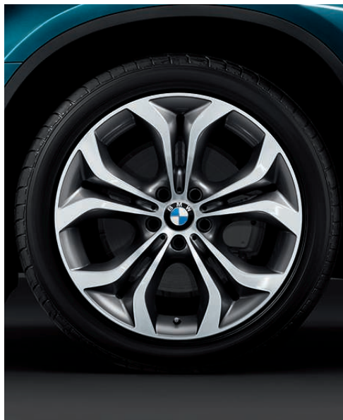
2LM 20" light alloy Y-spoke style 336 with mixed run-flat tyres , 10J x 20 with 275/40 R20 tyres at the front, 11J x 20 with 315/35 R20 tyres at the rear.
