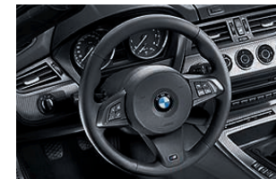
■ M Sport multi-function leather steering wheel: the extra thickness of the steering wheel ensures good grip. Integrated multi-function buttons allow the driver to operate the radio, CD player and optional Bluetooth telephone connection during a journey. Includes steering wheel mounted gearshift paddles in conjunction with automatic or Double Clutch Transmissions.
