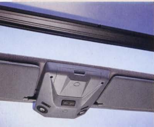
Electric slide and tilt glass sunroof with shade is standard on 'TR' level saloons.
