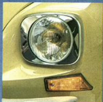
Headlamp beam level adjustable from inside the car.
