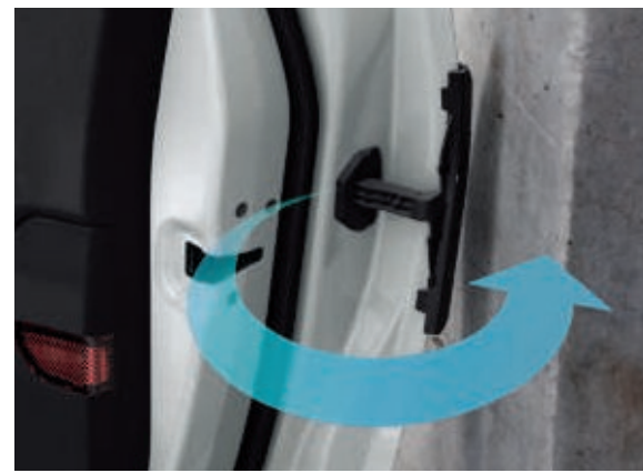
Retractable door edge protectors Activated when your vehicle doors are opened, the system helps to prevent undue damage by providing a protective barrier between your Fiesta Van's door edges and neighbouring parked vehicles or other obstacles.
