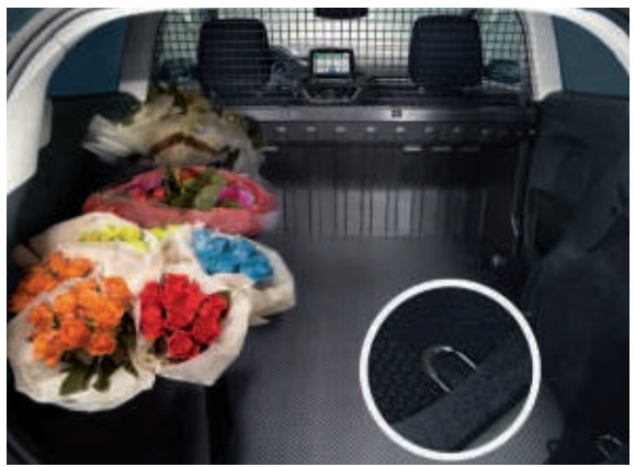
Ample load space Ford Fiesta Van offers a generous 0.96 cubic metres of rear load space. Four usefully placed tie-down points, plus a full load floor rubber mat, means you can transport items safely and securely without worrying about them moving around as you drive.
