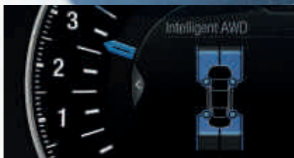
A special display on the cluster panel shows the power distribution between all four wheels. (Standard on all Intelligent All-Wheel Drive models)
