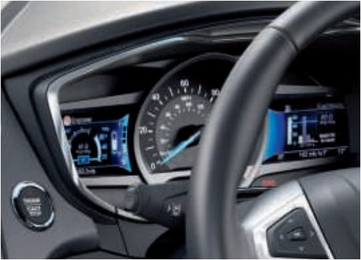
Twin 4.2" colour TFT cluster display with HEV SmartGauge®
