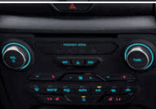
Dual-zone Electronic Automatic Temperature Control (DEATC) air conditioning (Standard)
