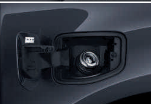
Ford Easy-Fuel capless refuelling system Prevents filling with the wrong fuel. (Standard)
