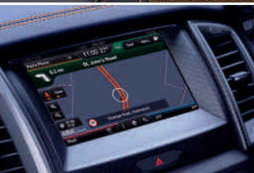
Ford SYNC 2 with 8" TFT touchscreen and Satellite Navigation (Standard)
