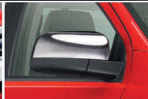
Power-operated and heated mirrors, chrome finish (Standard)
