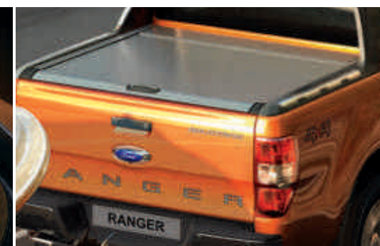
Lockable Integrated aluminium roller shutter (Option)
