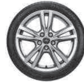
17" 5x2-spoke alloy wheel in Sparkle Silver-finish. Standard on Titanium
