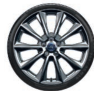
19" 10-spoke polished aluminium-finish alloy wheel Standard on Vignale (Fitted with 245/45 R19 tyres)
