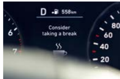
Driver Attention Alert (DAA) detects the onset of driver fatigue and provides both acoustic and visual alerts.
