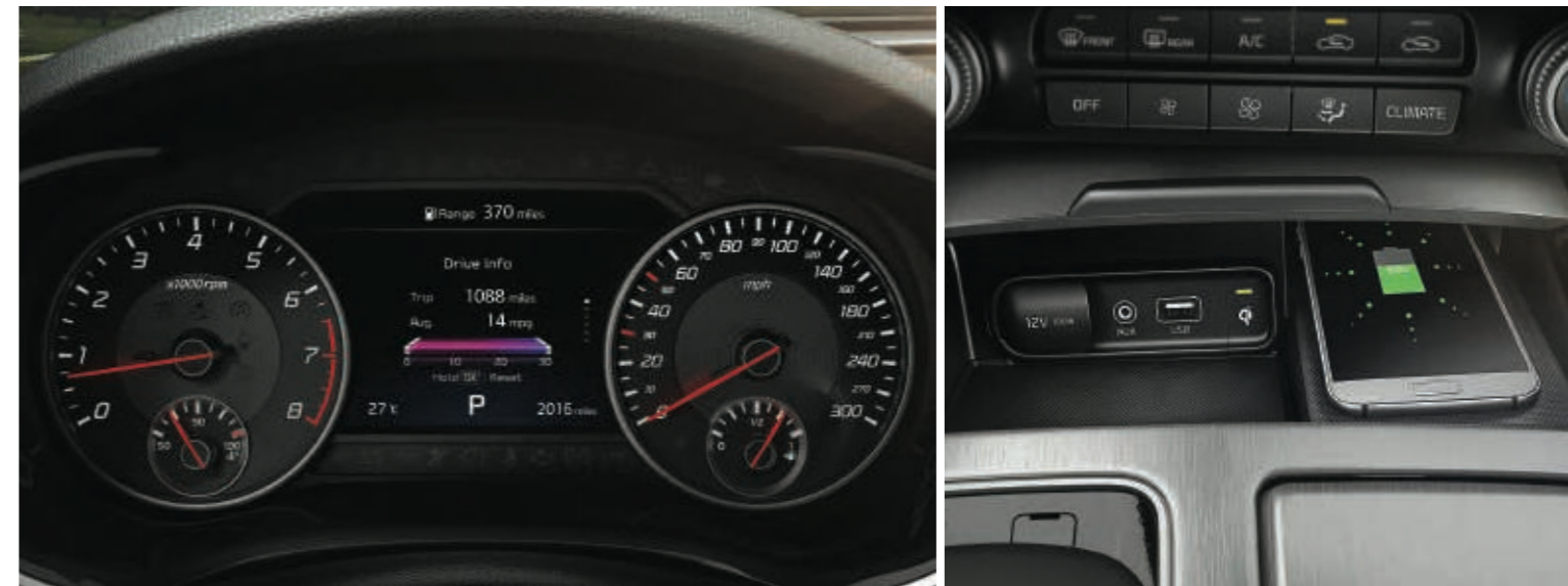
7" screen supervision cluster The high-definition 7-inch TFT LCD in the supervision cluster provides customisable data essentials - from average fuel economy to turn-by-turn navigation information.
