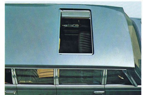
Sliding roof as fitted to 7-8 seat version
