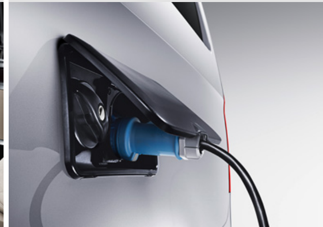
External connections for power and fresh water
