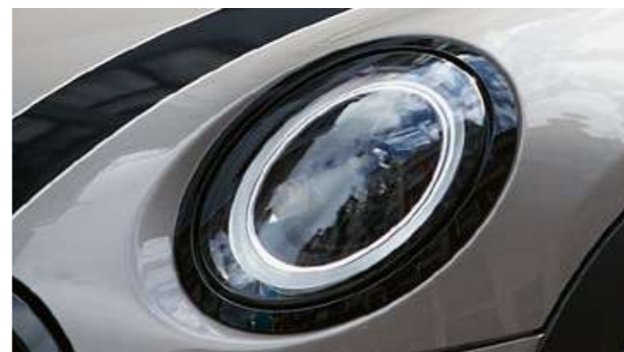
Adaptive LED headlights with Matrix function 9
