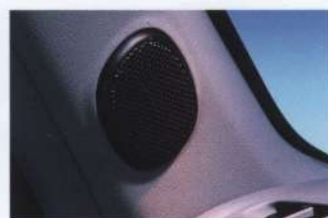
Audio tweeter in front pillar for enhanced sound reproduction.
