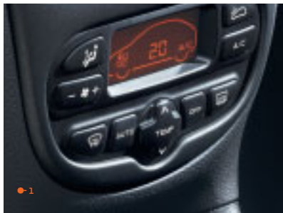
•-1 Digital air conditioning with climate control for control of the temperature and airflow. (On 2.0 SE model only – as standard)
