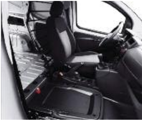
Multi-Flex retractable seat freeing up additional space
