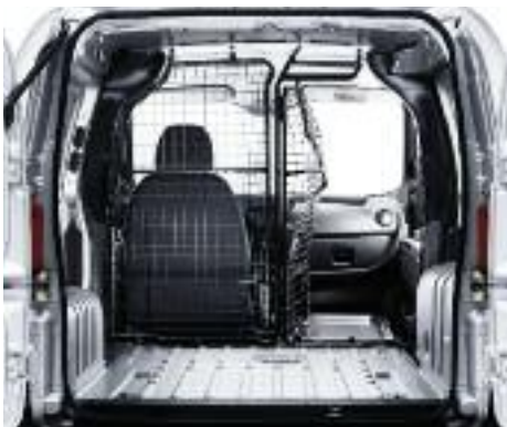
Modular partition linked with the retractable passenger seat**
