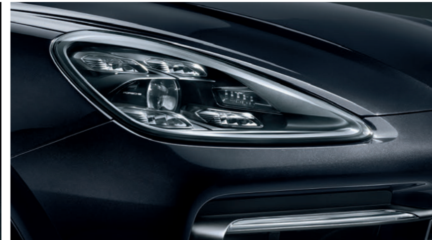
LED main headlights with matrix beam including PDLs Plus
