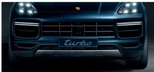
Skid plates in stainless steel
