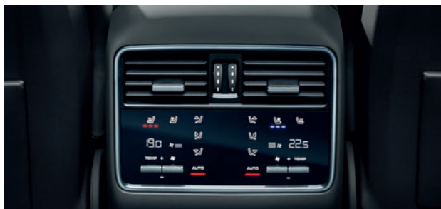
Four-zone automatic climate control
