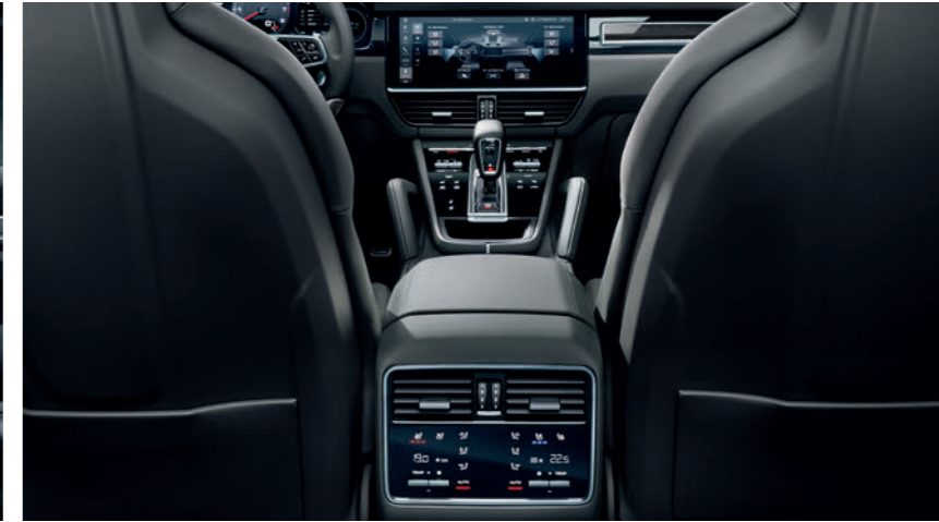
Four-zone automatic climate control
