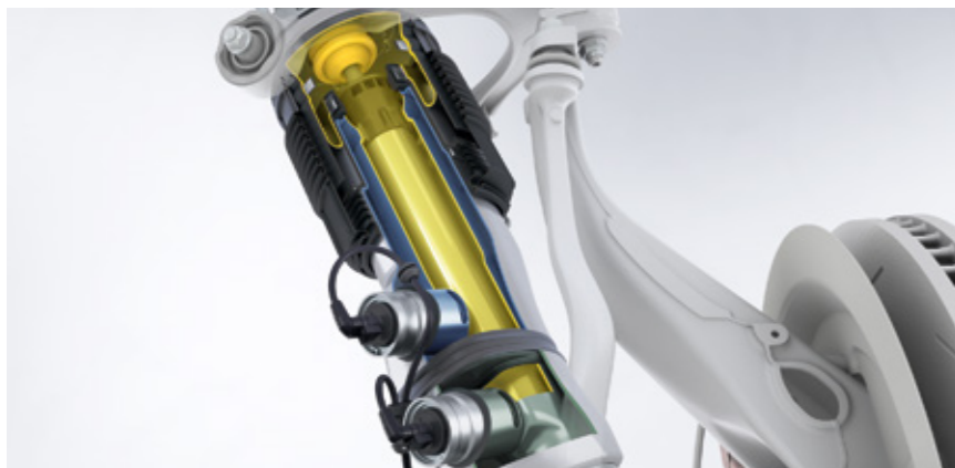
Adaptive air suspension with three-chamber technology
