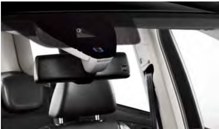
The multi-functional camera including Lane Assist and Traffic sign recognition (requires SEAT Media System and not available with heated windscreen).
