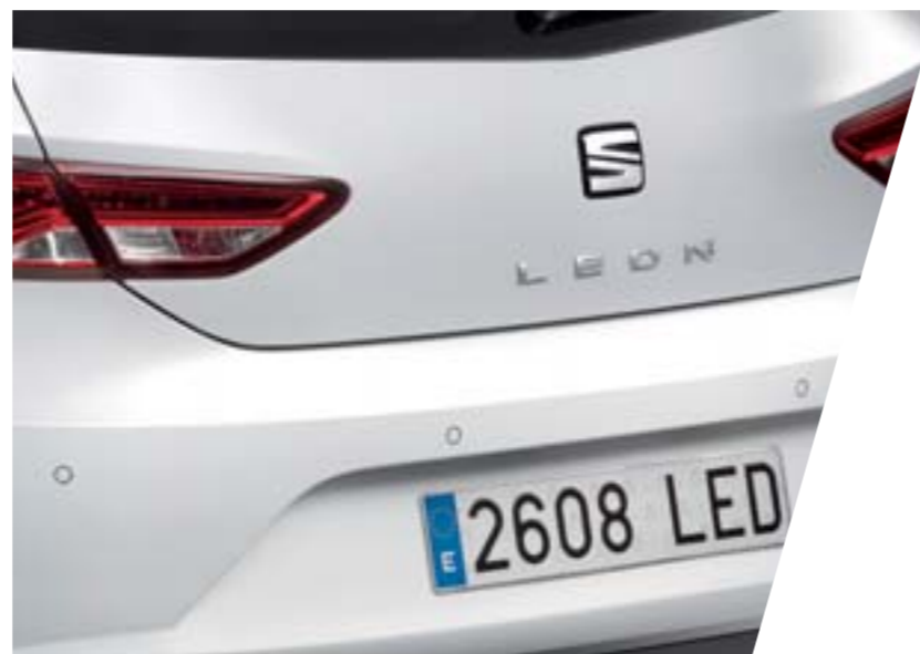
REAR PARKING SENSORS. Park with confidence and avoid any parking mishaps – full rear coverage from 160 cm to as close as 30 cm.
