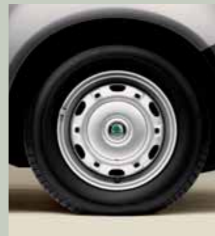
Steel wheels 5.0J x 13" with 155/80 R13 tyres. Standard for the Junior version.
