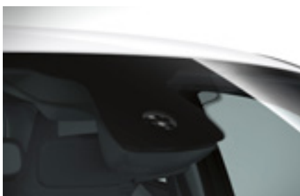
Rain/light sensor: rain sensor controls the windscreen wipers, adapting wipe intervals to amount of rainfall. The accompanying light sensor automatically activates driving lights
