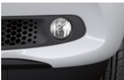
Fog lamps with cornering function
