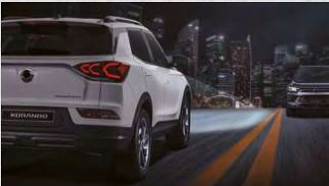
High Beam Assist Detects preceding vehicle's rear combination lights, headlights of oncoming vehicles and ambient brightness levels to automatically switch between high and low beams.
