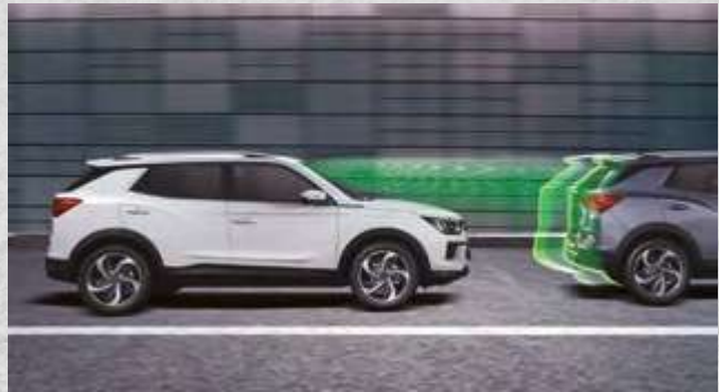
Front Vehicle Start Alert Alerts the driver when the preceding vehicle begins to depart.
