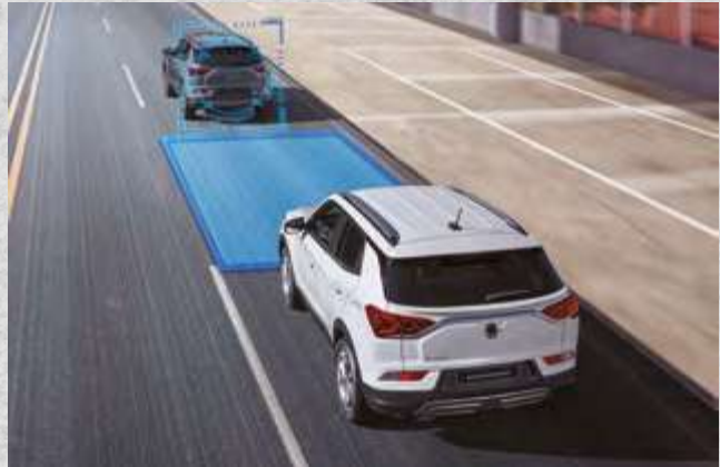
Safety Distance Alert The driver is alerted whenever a safe distance is not maintained from the preceding vehicle (the safety distance is automatically adjusted according to driving speed).
