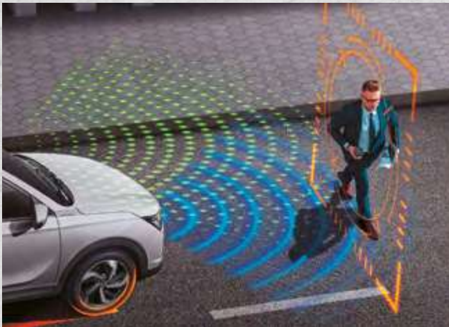
Front Collision Warning Alerts the driver when another vehicle or pedestrian appears in the path of the vehicle.
