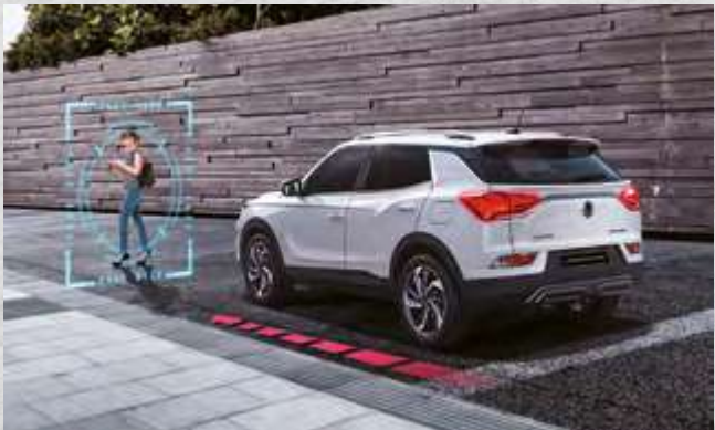
Autonomous Emergency Braking System When a frontal collision is anticipated, this function warns the driver and automatically applies the brakes to prevent a collision.
