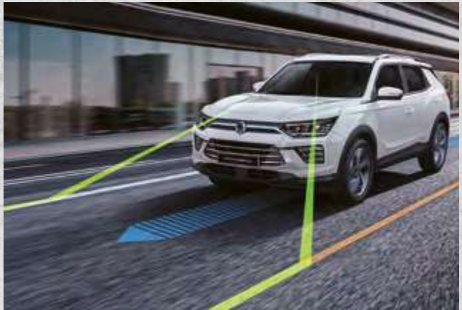
Lane Departure Warning System Notifies the driver when the forward camera module detects an unintended lane departure by the vehicle.
