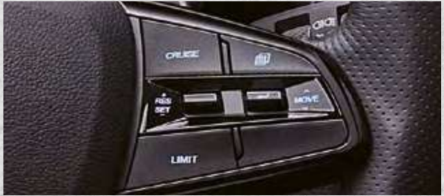
Cruise control Designed to be used on roads and motorways that don't have frequent stops and turns to negotiate, the electronic cruise control system enables the driver to hold a constant speed without driver input.
