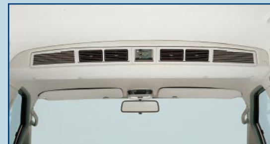
Overhead air conditioning, standard on the GX (not to UK specification)
