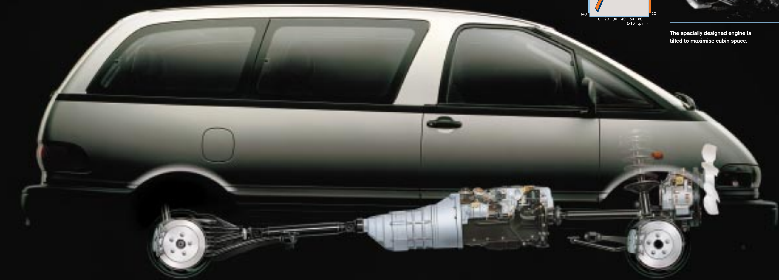
Innovative mid-engine layout creates a low centre of gravity producing car-like handling and road holding.
